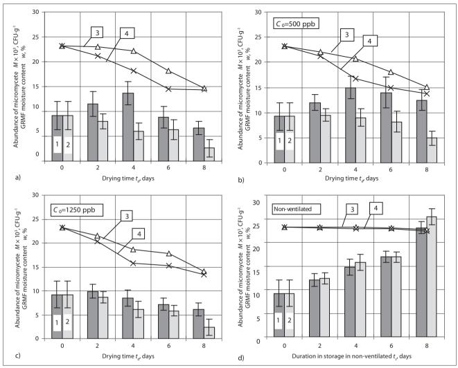
**Figure 6.** Changes of micromycete CFU in the active ventilation cylinder during the GRMF drying: 1 - CFU abundance in the top layers of raw material mound h = 1.0 m; 2 - CFU abundance in the bottom layers of raw material mound h = 0.20 m; 3 - the raw material moisture content of the top layers of the mound h = 1.0 m; 4 -GRMF moisture content in the bottom layers of the mound h = 0.20 m.
