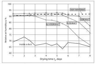
**Figure 3.** Impact of ventilation intensity on the relative humidity  $\phi$  changes in the top layer of the active ventilation cylinder with the wheat grain: the initial abundance of micromycete CFU in raw material of 23.2 ± 0.3% moisture content,  $M_n = 8.3 \times 10^3 \pm 1.5 \times 10^3 \text{ CFU} \cdot \text{g}^{-1}$
