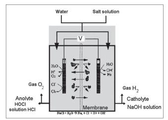
Figure 2. Device for electro-chemical activation of water [31]
