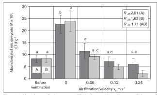
**Figure 4.** Abundance of micromycete CFU in the top (A) and bottom (B) layers of the active ventilation cylinder after 8 days of wheat raw material drying: the initial abundance of micromycete CFU at  $23.2 \pm 0.3\%$  moisture content of raw materials,  $M_0 = 8.3 \times 10^3 \pm 1.5 \times 10^3$  CFU·g<sup>-1</sup>.
